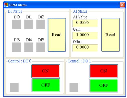
The function is used for controlling DO and reading the status of DIs and AI:
