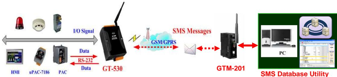
Before performing software installation, please configure GT-530/ GTM-201 hardware and set up the system (Figure above shows a possible system configuration. For more detail information, please refer to GT-530 User Manual.) Please be aware, The SMS Database System requires the .NET framework version 2.0 to be installed on the target computer. Please follow the link below to get the framework package directly from Microsoft, if required.
