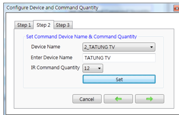
▲ Figure 3-11 Define the name and the quantity of the IR commands (Step2).
