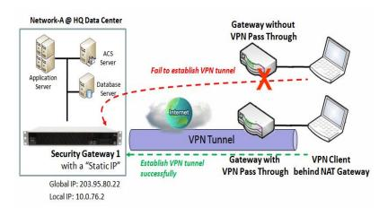
Since VPN traffic is different from that of TCP or UDP connection, it will be blocked by NAT gateway. To support the pass through function for the VPN connections initiating from VPN clients behind NAT gateway, the gateway must implement some kind of VPN pass through function for such application. The gateway support the
