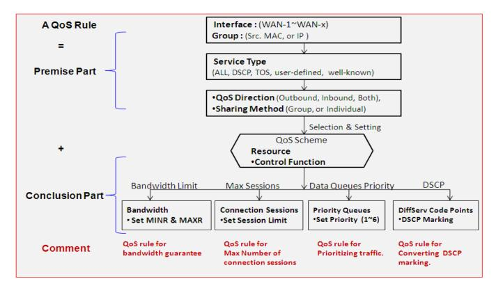
In above diagram, a QoS rule is organized by the premise part and the conclusion part. In the premise part, you must specify the WAN interface, host group, service type in the packets, packet flow direction to be watched and the sharing method of group control or individual control. However, in the conclusion part, you must make sure which kind of system resource to distribute and the control function based on the chosen system resource for the rule.
