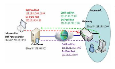
As shown in the diagram, Gateway has the IP address of 118.18.81.200 for WAN interface and 192.168.1.253 for LAN interface. It serves as a NAT gateway. Users in Network-A initiate to access cloud server through the gateway. Sometimes, unknown users will simulate the packets but use different source IP to masquerade. With the SPI feature been
