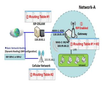
The Routing Information Protocol (RIP) is one of the oldest distance-vector routing protocols, which employs the hop count as a routing metric. RIP prevents routing loops by implementing a limit on the number of hops allowed in a path from the source to a destination. The maximum number of hops allowed for RIP is 15. This hop limit, however, also limits the size of networks that RIP can support. A hop count of 16 is considered an infinite distance, in other words the route is
