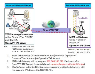
The term "TAP" is referred to bridge mode and operates with layer 2 packets. In bridge mode, the VPN client is given an IP address on the same subnet as the LAN resided under the OpenVPN server. Under such configuration, the OpenVPN client can directly access to the resources in LAN. If you want to offer remote access to the entire remote LAN for VPN client(s), you have to setup OpenVPN in "TAP" bridge mode.
