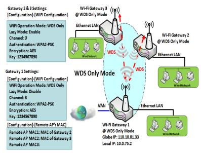
This mode allows you to get your wired and wireless devices connected to form the Intranet of the wireless gateway, and the Intranet will link to the Internet with NAT mechanism of the gateway. So, this gateway is working as a WiFi AP, but also a WiFi hotspot for Internet accessing service. It means local WiFi clients can associate to it, and go to Internet. With its NAT mechanism, all of wireless clients don't need to get public IP addresses from ISP.
