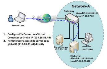
"Virtual Computer" allows you to assign LAN hosts to global IP addresses, so that they can be visible to outside world. While so, they are also protected by the gateway firewall as being client hosts in the Intranet. For example, if you set a FTP file server at LAN side with local IP address 10.0.75.102 and global IP address 118.18.82.44, a remote user can access the file server while it is hidden behind the NAT gateway. That is
