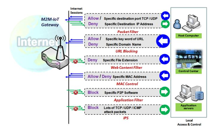
The firewall functions include Packet Filter, URL Blocking, Content Filter, MAC Control, Application Filter, IPS and some firewall options. The supported function can be different for the purchased gateway.
