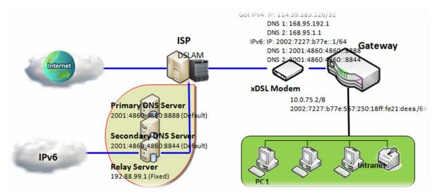
In above diagram, the 6to4 means no need to set gateway address "automatic" tunneling solution. The automatic mean have relay server, as defined in RFC 3068 has included segments draw 192.88.99.0/24 used as 6to4 relay of any-cast address to complete 6in4 setting. 6in4
