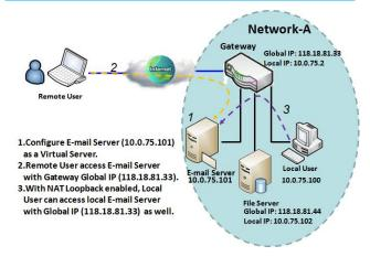
"Virtual Server" allows you to access servers with the global IP address or FQDN of the gateway as if they are servers existed in the Internet. But in fact, these servers are located in the Intranet and are physically behind the gateway. The gateway serves the service requests by port forwarding the requests to the LAN servers and transfers the replies from LAN servers to the requester on the WAN side. As shown in example, an E-mail virtual
