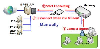
**Manually:** This gateway won't start to establish WAN connection until you press "Connect" button on web UI. After normal data transferring between LAN and WAN sides, this gateway will disconnect WAN connection if idle time reaches value of Maximum Idle Time.
