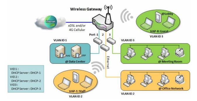
Above is the general case for 3 Ethernet LAN ports in the gateway. But if the device just has one Ethernet LAN port, there will be only one VLAN group for the device. Under such situation, it still supports both the NAT and Bridge mode for the Port-based VLAN configuration.
