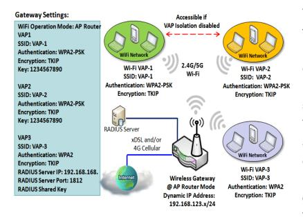
VAP (Virtual Access Point) is function to partition wireless network into multiple broadcast domains. It can simulate multiple APs in one physical AP. This wireless gateway supports up to 8 VAPs. For each VAP, you need to setup SSID, authentication and encryption to control Wi-Fi client access.
