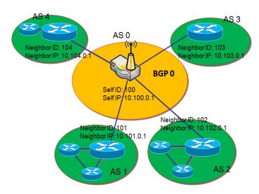
Border Gateway Protocol (BGP) is a standard exterior gateway protocol designed to exchange routing and reachability information between autonomous systems (AS) on the Internet. It usually makes routing decisions based on paths, network policies, or rule-sets. Most ISPs use BGP to establish routing between one another (especially for multihomed). Very large private IP networks also use BGP internally. The major BGP gateway
