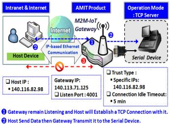
Terminate this TCP Connection once Idle Timeout reached 5 mins.
