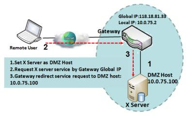
When the network administrator wants to set up some service daemons in a host behind NAT gateway to allow remote users request for services from server actively, you just have to configure this host as DMZ Host. As shown in the diagram, there is an X server installed as DMZ host, whose IP address is 10.0.75.100. Then, remote user can
