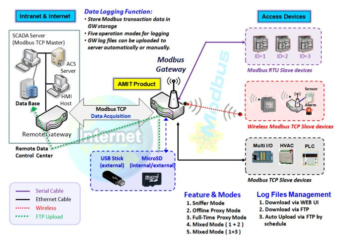
The Modbus Cellular Gateway provides a complete data logging function for collecting the
