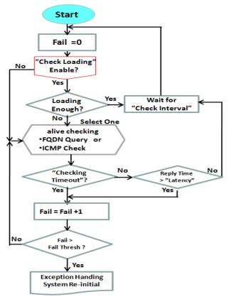
It is necessary to monitor connection status continuous. To do it, "ICMP Check" and "FQDN Query" are used to check. When there is trafiic of connection, checking packet will waste bandwidth. Response time of replied packets may also increase. To avoid "Network Monitoring" work abnormally, enabling "Checking Loading" option will stop connection check when there is traffic. It will wait for another "Check Interval" and then check loading again.
