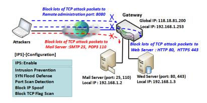
As shown in the diagram, the gateway serves as an E-mail server, Web Server and also provides TCP port 8080 for remote administration. So, remote users or unknown users can request those services from Internet. With IPS enabled, the gateway can detect incoming attack packets, including the TCP ports (25, 80,
