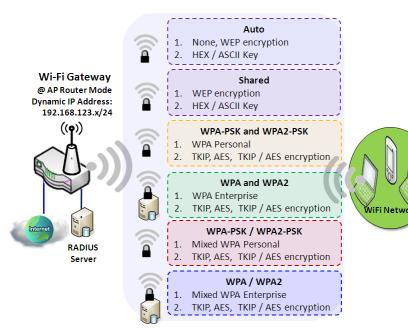
Wi-Fi security provides complete authentication and encryption mechanisms to enhance the data security while your data is transferred wirelessly over the air. The wireless gateway supports Shared, WPA-PSK / WPA2-PSK and WPA / WPA2 authentication. You can select one authentication scheme to validate the wireless clients while they are connecting to the AP. As to the data
