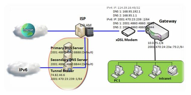
In above diagram, the 6in4 usually needs to register to a 6in4 tunnel service, known as Tunnel Broker, in order to use. It also need end point global IPv4 address as 114.39.16.49 to complete 6in4 setting.
