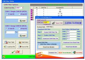
This utility configures the CAN filter and user-defined CAN baud rate. It can save the CAN filter configuration as file and would be import to another I-2534 or I-5534-M.
