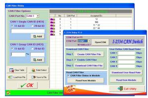
This utility configures the CAN filter and user-defined CAN baud rate. It can save the CAN filter configuration as file and would be import to another I-2534.
