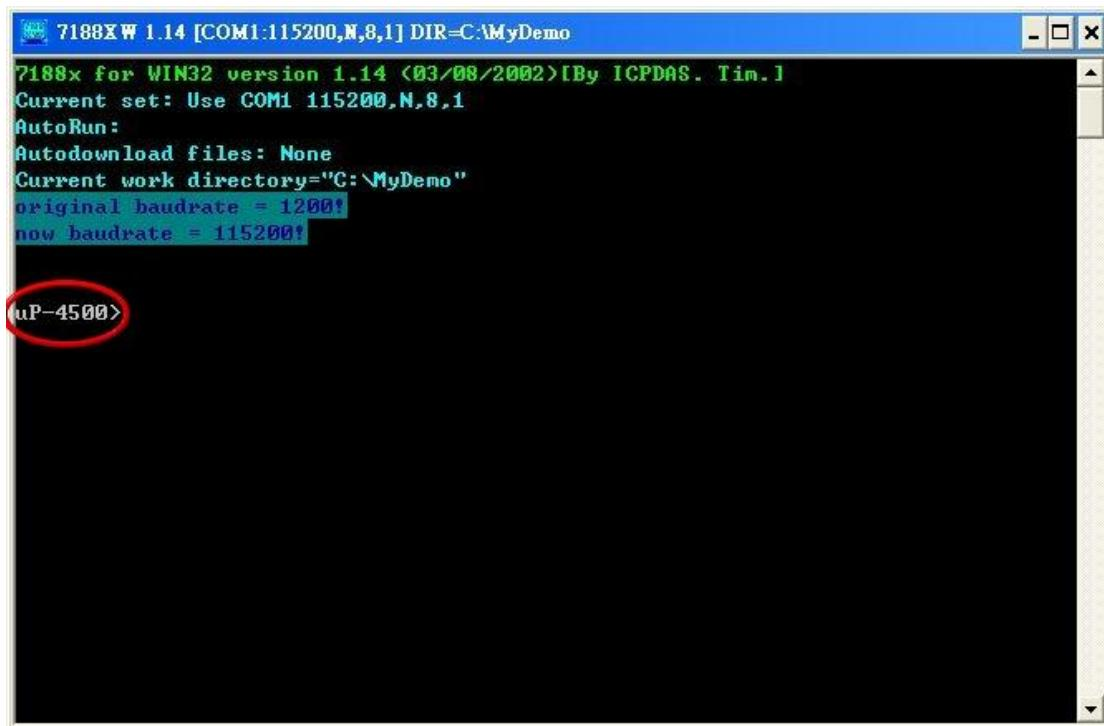
Step 10 : Key the command, “load” in the 7188xw.exe program. Then, follow the hint command to press “Alt+E” and input the file name, “TEST.exe” , to download the execution file.
